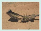
The weeders that are available in the market are a bit costly. There are some problems with the design also. When these are being used in heavy soils, there are several problems. Different weeders were studied and by combining the advantages of each one, a new 'mandava' weeder has been designed The weeder got its name after 'Chinna Mandava', a village in Khammam district in Andhra Pradesh, where it has been tested and fine tuned.
