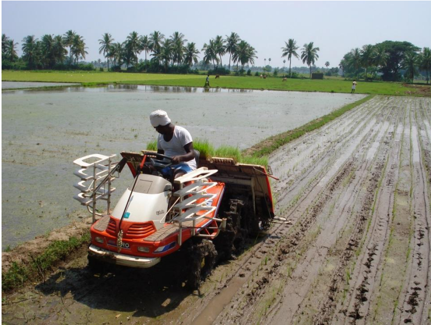
Mechanized SRI transplanting, Tamil Nadu
